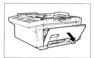
3. Swing down the toner cartridge by pulling it down from the top. Then remove the cartridge from the development unit.
